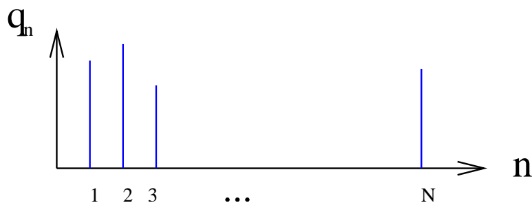
Fig. 1. Like other MC methods, KMC must repeatedly sample from discrete distributions/ensembles. For KMC, this distribution corresponds to a list of rates \{q_n\} that typically changes from one time-step to the next and a corresponding set of events \{\Delta X_n\} that represent local changes to the system state.
