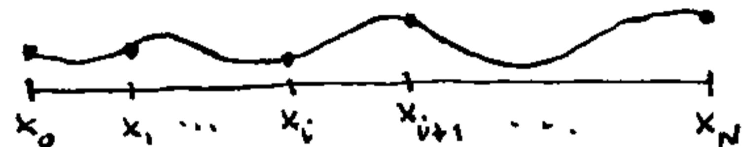
$$S(x) = S_i(x) \text{ on } [x_i, x_{i+1}] \quad i=1, \dots, N-1$$
