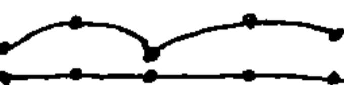
piecewise cubic: a cubic on  $\{x_i, x_{i+1}, x_{i+2}, x_{i+3}\}$
